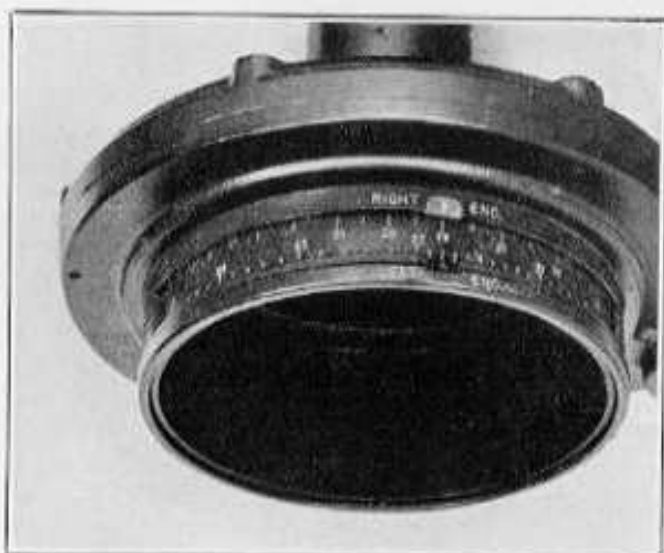
Fig. E 492b. Detail of Wavelength Range Drum.
