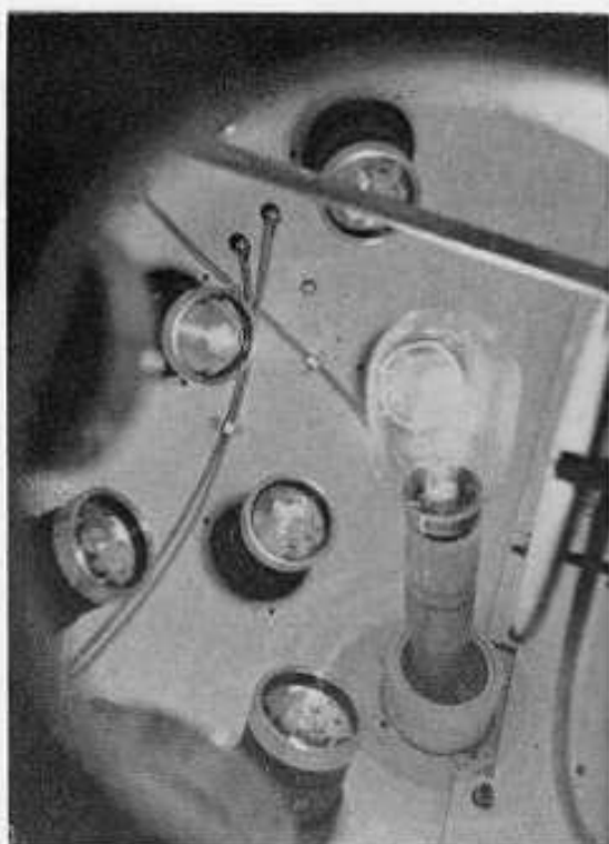
Inner Side of Fixed Star Projectors Globe. (Projector Lamp and Condensers.)
