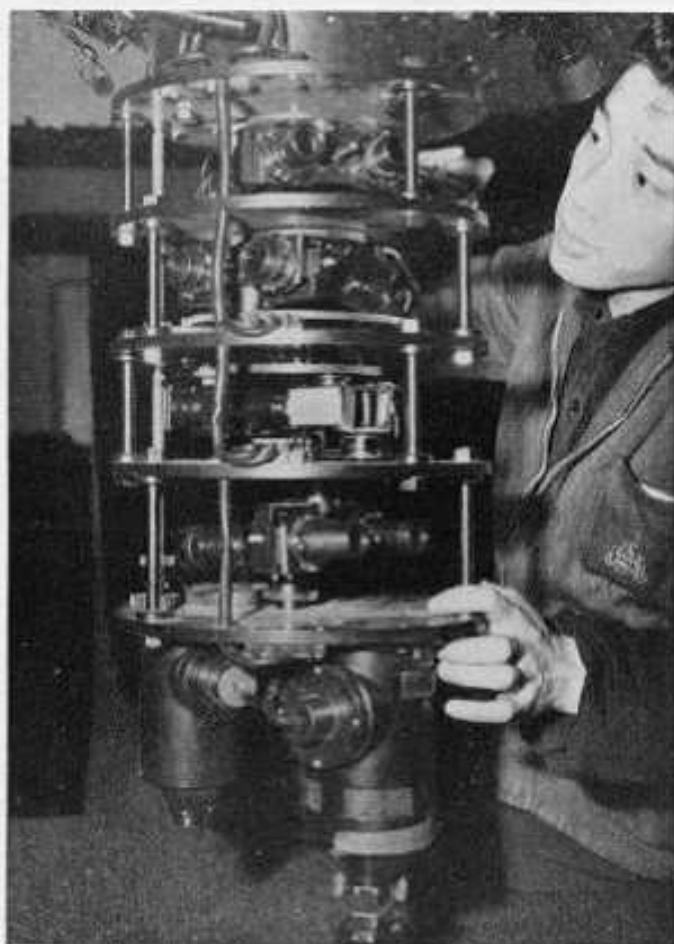
Planet Projectors Mechanism.
