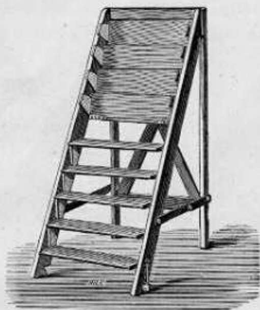
Simple Observing Chair, with Movable Steps.
