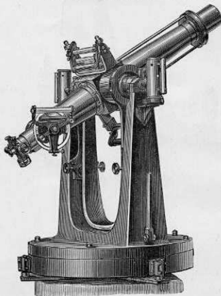
Transit Instrument, with Reversing Arrangement and Two Setting Circles.
