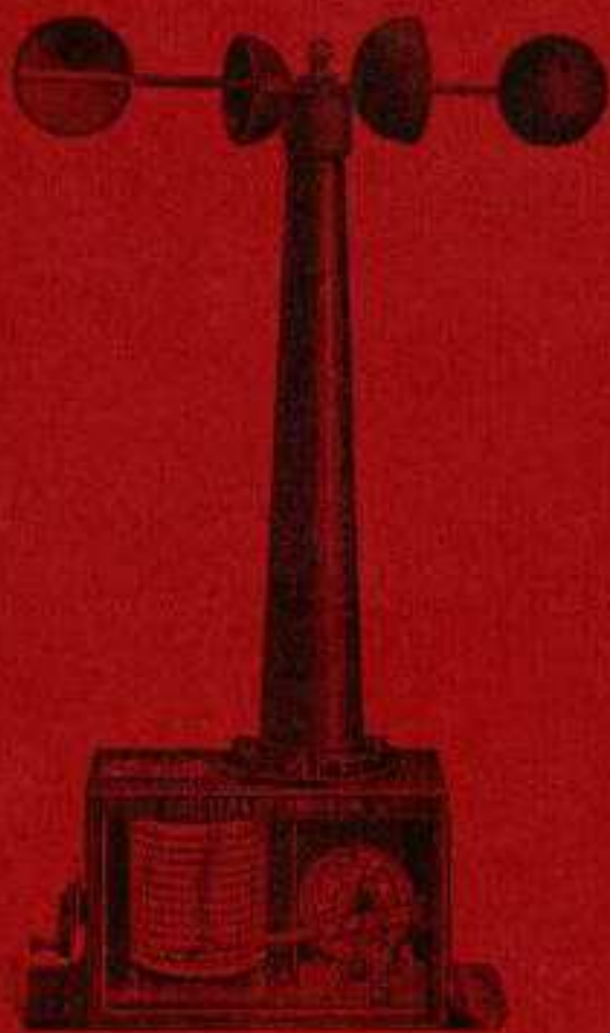
C. F. CASSELLA'S PATENT ANEMOMETER. DIRECT READING AND RECORDING.
